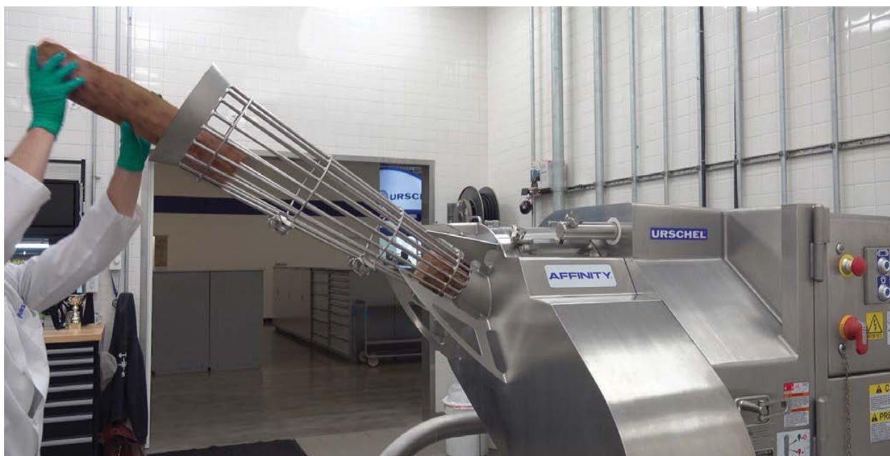
The Affinity Pre-Cutter has a built-in pre-cutter for the processing of logs
