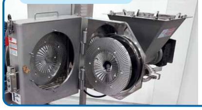
Product texture is controlled via the plate gap adjustment
