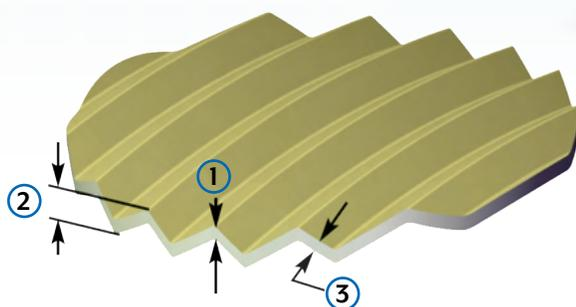
The Z-Cut slice can be produced in thicknesses from .030" to .115" (0.8 to 2.9 mm). Slice thickness is measured at the peak [1]. Overall slice thickness [2] and the thickness of the angled side or flank [3]. The shorter flank is the thinnest section of the slice. The corrugations [4] are .135" (3.4 mm) deep and measure .394" (10 mm) from peak to peak. There are 2.54 corrugations per inch (25.4 mm).
