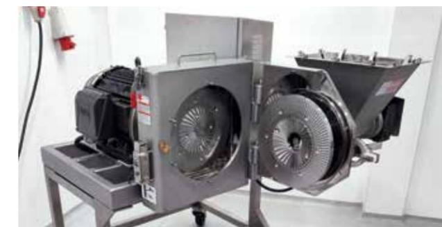
Product texture is controlled through the type of plates used and the gap adjustment
