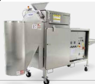
The TranSlicer® 2510 Cutter is the precursor to the new 2520. Both machines offer the same styles of 25" (635 mm) cutting wheels. To accommodate different products, customers have a choice between three different feed belt configurations: primary belts only, primary and secondary belts, or full-length primary belts. The machine operates via a VFD (variable frequency drive).
