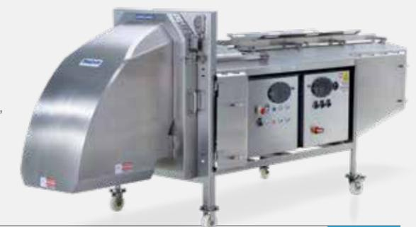
**The CC Slicer features interchangeable cutting heads.** MicroAdjustable® Slicing (SL-14), Shred (SH-14), and Julienne Heads feature 14 cutting stations with expedited maintenance. The cutting chamber, surrounding the cutting head, is available in a 22" (559 mm) or 32" (813 mm) diameter. New frame design delivers increased sanitation and flexibility.
