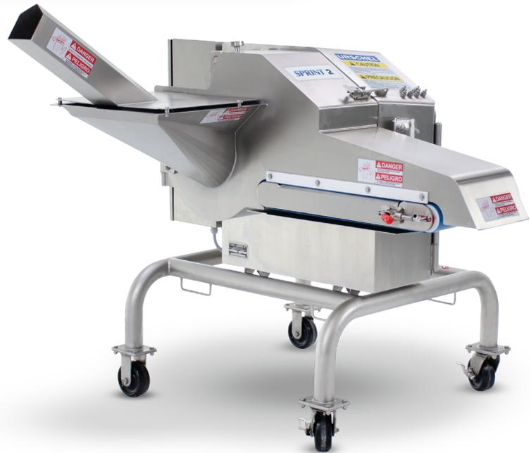
Under development for the Sprint 2 Dicer, the new feed chute offers precision delivery of products such as jumbo carrots. Cutting applications include carrot sticks and batons. By increasing feeding accuracy, a larger percentage of infeed product engages with the cutting parts to increase yield. Streamlined processing increases overall cost-savings maximizing time and the amount of cut product within the desired target range.
