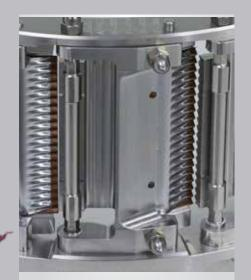
Adjustable gate flexes as top/ bottom adjustable cams are turned to provide microadjustability of shred thickness.
