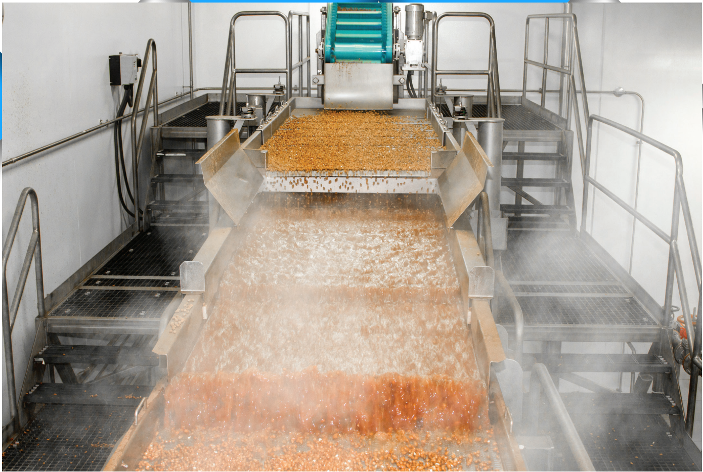
Almonds emerge for blanching on this line. Wet and dry process steps are sequential and separate in this facility.
