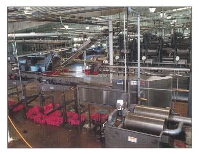
With the **TranSlicer** 2000, product is delivered onto high-speed feed belts sloping together to form a Vshaped feed trough. The two feed belts are synchronized with a 20-in.diameter rotating slicing wheel to ensure proper advance of product- in this case asparagus.
