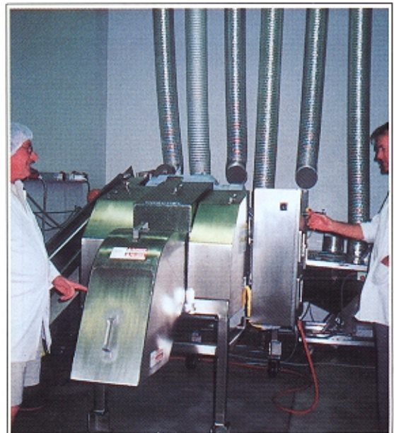
Below: The Urschel cutting machine from Nuritur has enabled TropiCube to develop a wide range of product sizes and shapes.
