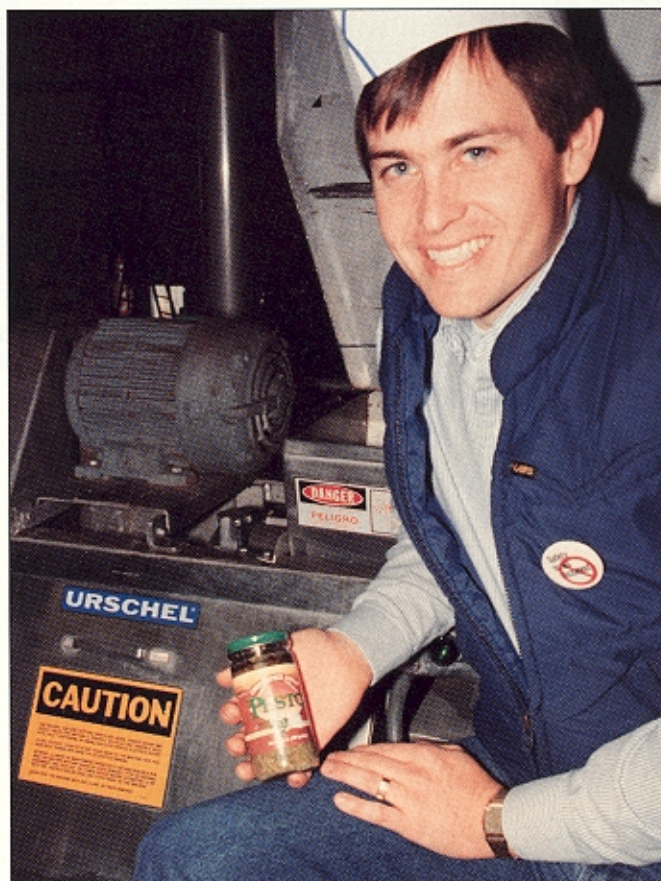
Fresh basil and parsley is run through an Urschel milling machine that cuts the product into a specific particle size, a benefit noted by Jim Wallace, Christopher Ranch production engineer.
