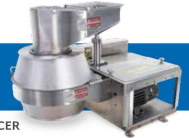
Lattice slicing is a unique application. Proper feeding of the machine is necessary to ensure continuous production. Tempered high quality oval or flat shaped potatoes measuring between 2 to 4 inches (51 to 102 mm) are best-suited. Model CC Slicers can be converted to Model CCL Lattice Slicers.
