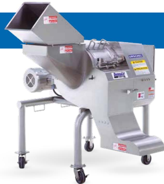
**Designed with cutting zone completely separate from the mechanical zone.** Rounded tube frame contributes to sanitary design and eases cleaning. Provides slicing-only capability and 2- or 3-dimensional cutting for a full range of dices, crumbles/granulations, or strips. A variety of shreds are also available.
