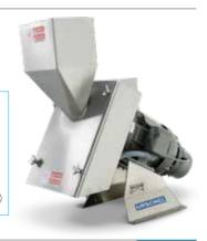
The Model 1500 utilizes Microcut 6" (152.4 mm) diameter style reduction heads. Recommended for specific applications where refining or finishing of free-flowing liquids or viscous slurries is desired
