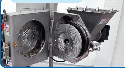
Product texture is controlled through the type of plates used and the gap adjustment
