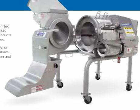
Cutting zones are completely separate from mechanical zones. Rounded tube frame contributes to sanitary design and eases cleaning.
