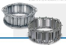
MicroAdjustable® SH-14 & SL-14 heads offer increased capacity with 14 cutting stations versus the standard 8 head. To determine the availability of specific thicknesses and styles, visit www.urschel.com.
