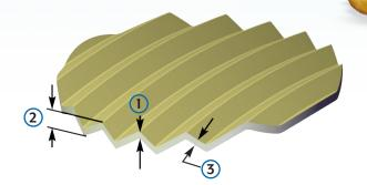
The Z-Cut slice can be produced in thicknesses from .030" to .115" (0.8 to 2.9 mm). Slice thickness is measured at the peak [1]. Overall slice thickness [2] and the thickness of the angled side or flank [3]. The shorter flank is the thinnest section of the slice. The corrugations [4] are .135" (3.4 mm) deep and measure .394" (10 mm) from peak to peak. There are 2.54 corrugations per inch (25.4 mm).
