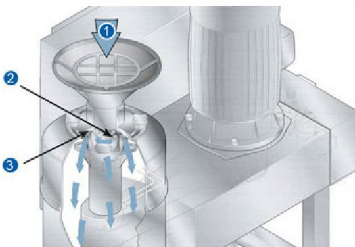
Fig.3: A versatile comminution mincer/slicer
