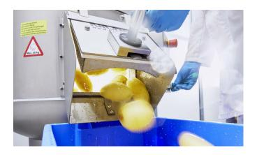
The filling and peeling process can be controlled centrally by means of an automatic control system (optional). The PL 25K can therefore be ideally integrated into complete processing lines for the washing, peeling and cutting/dicing of root vegetables.
