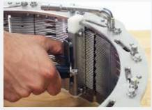
Flat slice setup features quick-release clamps, positive cam opening, and handled knives.
